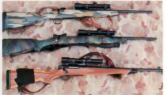
An assemblage of early Scout Rifles, including (top to bottom): Scout VI, built on a Czech ZKK 601 short action in .308 Winchester; Scout X, built with a Winchester Model 70 short action of current manufacture and chambered for the .308 Winchester round; and Super Scout I with a Remington 660 action chambered for the .350 Remington Magnum cartridge.
